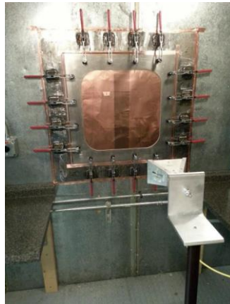
Example of how to do the IEEE-299 test correctly (with seams and tape)
