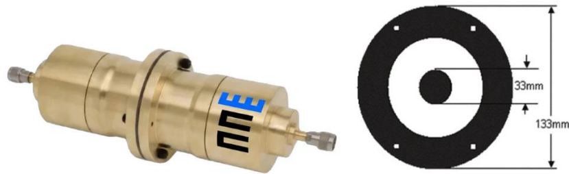
Example of an ASTM D4935 Test Setup
