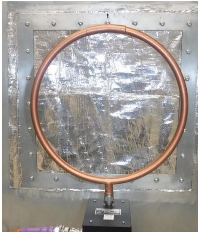
Example of how NOT to do the IEEE-299 test (no seams & no tape)
