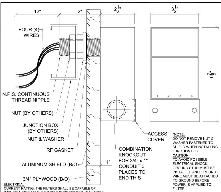
WITHSTANDING 140 % OF RATED CURRENT FOR 15 MINUTES WITHOUT ANY DETERIORATION.
