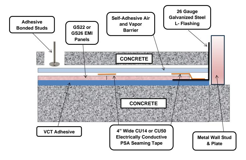
4" x 4" or 6" x 6" 26 Gauge Galvanized Steel L- Flashing is Typical Wall Shielding Attaches to the Vertical Portion of the Flashing
