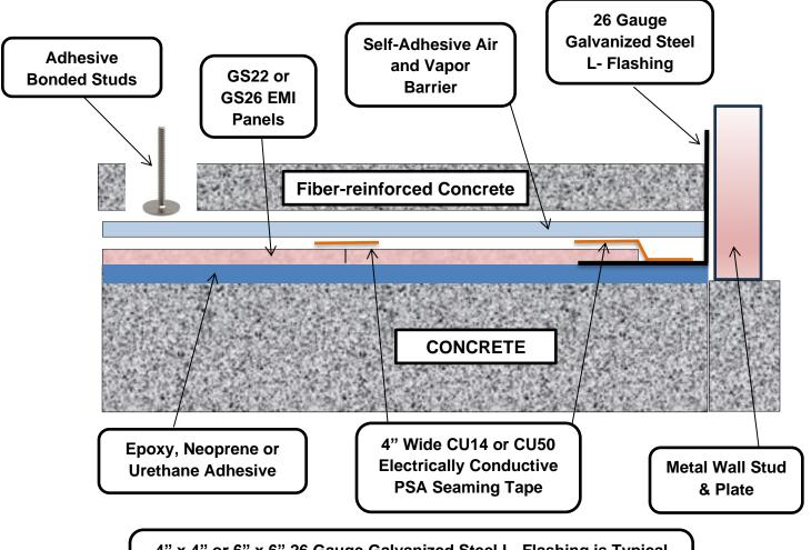
4" x 4" or 6" x 6" 26 Gauge Galvanized Steel L- Flashing is Typical Wall Shielding Attaches to the Vertical Portion of the Flashing
