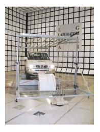
The TDK STL-03 Stripline generates electric fields over the frequency range of DC-30 MHz, and is designed for radiated immunity testing of automotive and aircraft equipment.
