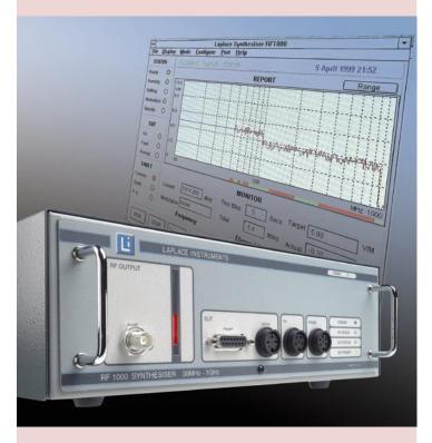
**EUT MONITORING.** Real time monitoring and logging of EUT status facilitates accurate recording of test progress and reporting. Flexible EUT status response modes allow unattended testing for greatest productivity.
