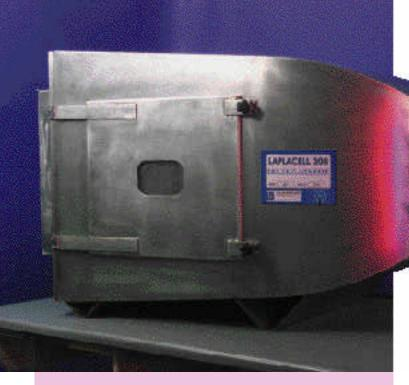
The LaplaCell is the result of an extensive R & D programme to provide a solution to the particular problems facing organisations who wish to self test products for EMC compliance. The unique design features a novel double tapered internal profile which provides a very compact cell with a built-in field sensor. Each cell is individually characterised for field strength vs sensor output and emissions sensitivity so that results can be correlated against an OATS.
