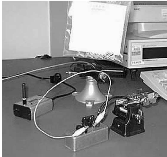
Fig. 10. ESD source and loop antenna.
