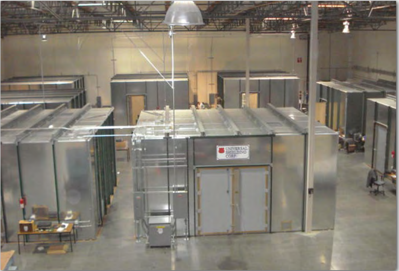
Complex consisting of nine shielded anechoic enclosures. Installed at DNB Engineering, Inc. Fullerton, CA.
