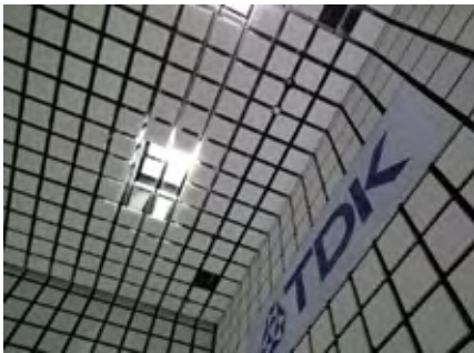
You can not see the lighting fixtures even when you are close to them. This is the basic principle of wave reflection prevention.
