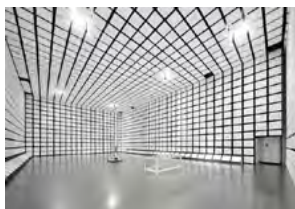
L25m x W14m x H9m Absorber: IP-130BLB(H:1300mm) ANSI: ±3.0dB VCCI: ±1.5dB
