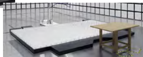
Installation of panel with bsorbers is completed.
