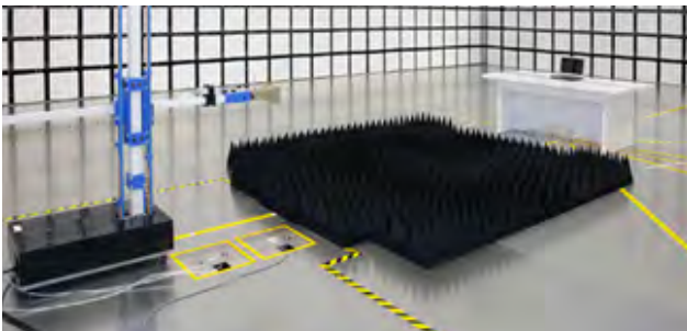
Antenna evaluation anechoic chamber (800MHz to 110GHz): Installing the electromagnetic wave absorber IS-030A on the floor between radiation antenna and EUT (equipment under test) (25 units of 3*3m in this case) can significantly reduce reflected waves from the floor and achieve the Site VSWR standard (SVSWR: 6dB or lower).
