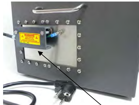
STEFILT24 INSTALLED ON I/O PLATE
